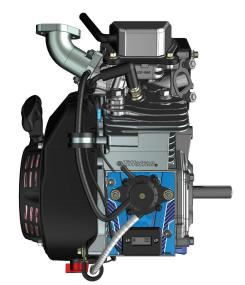
Note: Black Fuel Line represents the Pulse Connection from the fuel pump to the intake manifold connector.
